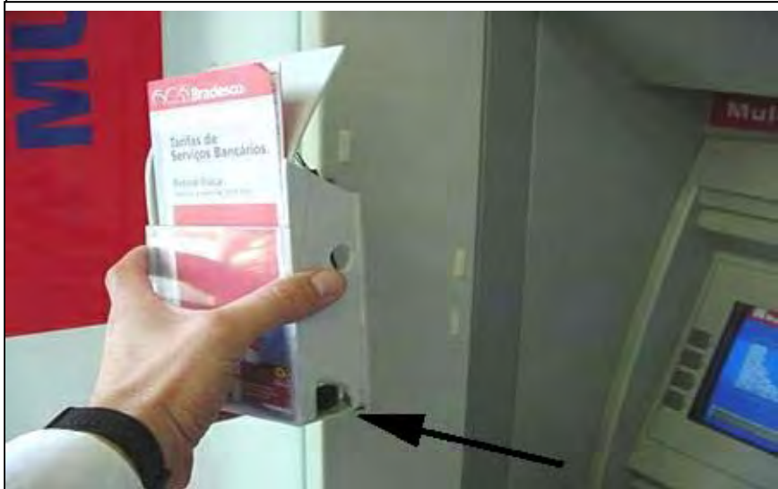
The PIN reading camera, housed in an innocent looking leaflet container.
