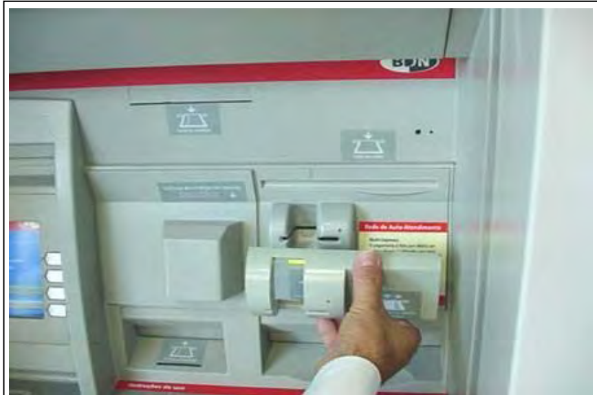
The card skimmer, showing its installation in front of existing card slot.
