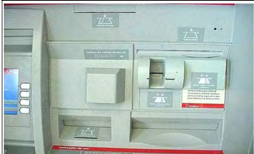
The card skimmer as it appears installed
